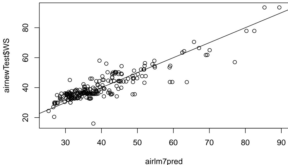
As seen from the summary results, model 3 contained an adjusted R squared of .98 and a residual standard error of 5.581. Both explanatory variables contained significant P values. The predicted vs actual plot resembles a linear structure that closely follows the plotted abline. As wing span increases, more variance in the predicted values can be seen. The residual vs fit, and normal qq plots can be seen in the appendix of the paper.
